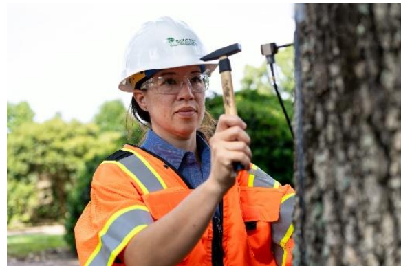
Figure 1: When using sonic tomography, arborists tap sensors to send soundwaves through a tree.
