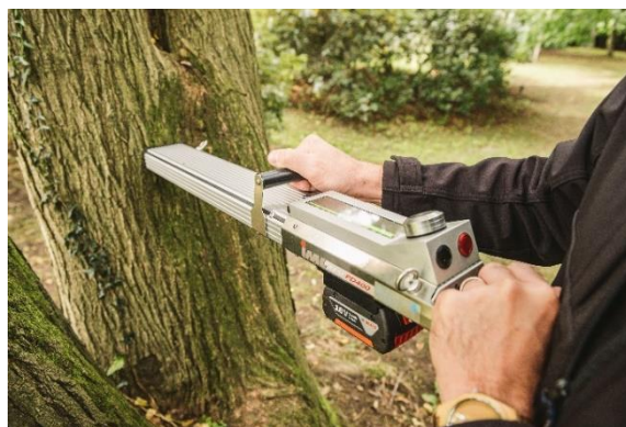
Figure 4: Resistance drills use small drill bits to record resistance within a tree.
