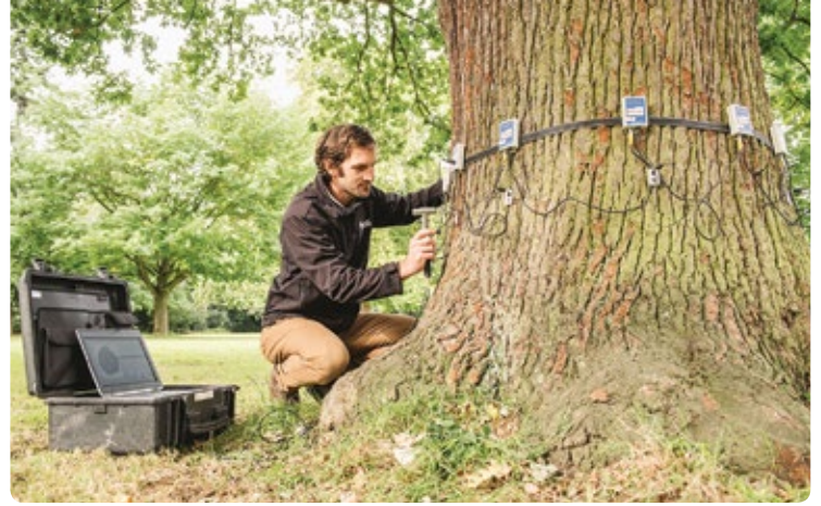
A Bartlett arborist assessing the interior of a tree with a PiCUS sonic tomograph.
