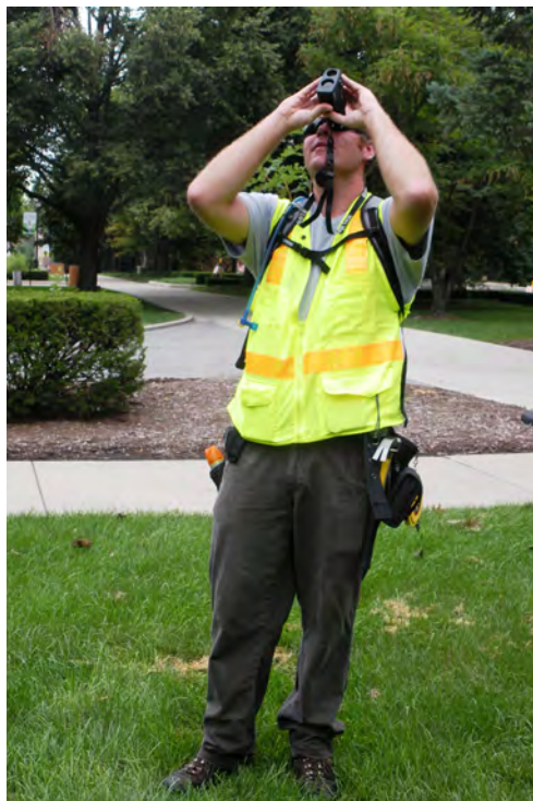
A laser device measures tree height.
