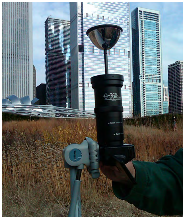
A 360-degree panoramic camera used to document trees in Chicago's Millennium Park as part of the BIS inventory and management plan. The images can also be used to provide a virtual tour of the world-famous park.
