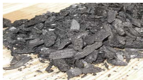
Figure 1: Biochar made from wood chips of pine trees killed by Mountain Pine Beetle
